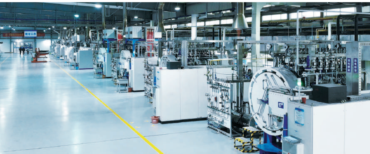
Sintering of inserts
