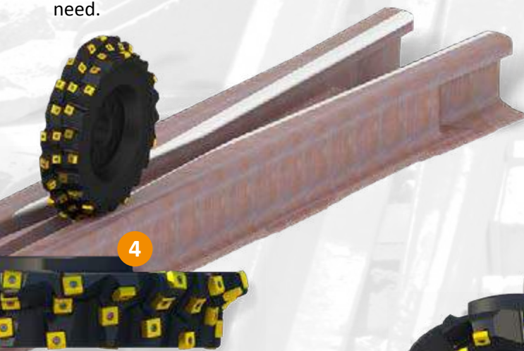
4 – Disc milling cutter for machining of the top of the rail head ø 350 mm, machining of corner radius (R13) and the side of the head in the groove. Protective inserts in the biggest cutter diameter in case of extra material removal need.
