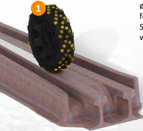
2 – Concave style milling cutter for machining of the wing rails maximum ø 340 mm with very wide cutting area for milling of corner radius (R13), top radii (R80, R300) and two inclined faces (1:20, 1:10).
