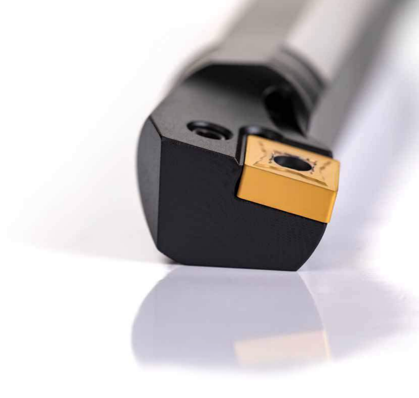
TCMT 110204E-NF1:T9325 NF1 geometry with positive design for fine-finish to semi-rough machining in stainless steel and superalloys, also suitable for steel, hardened materials and non ferritic materials. For continuous machining.
