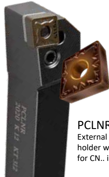
CNMG120408E- FM:T8430 FM geometry with positive design for fine-finish to semi- rough machining in steel, stainless steel and cast iron, and superalloys in continuous and slightly inter- rupted machining.
