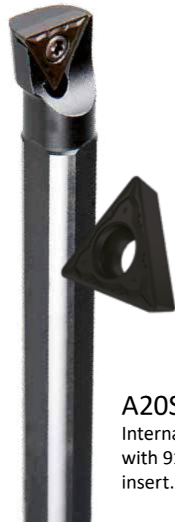
TCMT 110204E-NF1:T9325 NF1 geometry with positive design for fine-finish to semi-rough machining in stainless steel and superalloys, also suitable for steel, hardened materials and non ferritic materials. For continuous machining.
